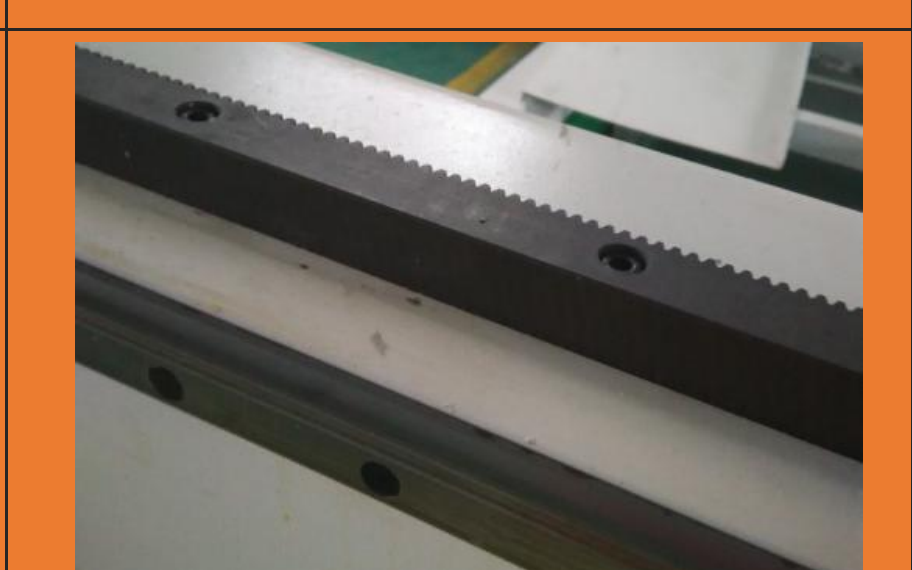
square rail, rack transmission
